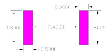
**♦ 2<sup>nd</sup> Layout Dimensions in Clearance area**(Size=8.0\*3.0mm)
